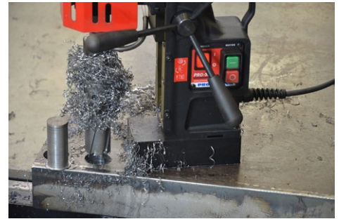
Milling capacity up to 45 mm (2") Depth of cut up to 75 mm (3") - option
