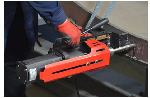
Drilling capacity up to 18 mm (0.71")
