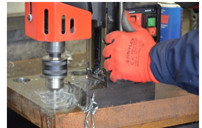
Drilling capacity up to 16 mm (0.63")
