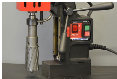
TCT cutters up to \Phi 45 mm with AMT2-C19/2-3 arbor D.O.C. up to 75 mm
